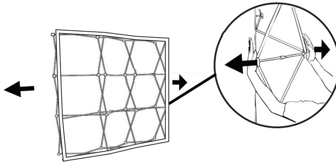
3. Once the frame has expanded fully push the two sides of a hook on each cross section so that you can hook the frame secured firmly in place.
