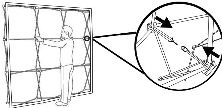
4. Repeat steps 1-3 to assemble the second half of the backwall. Attach the graphic print to the velcro frame.
